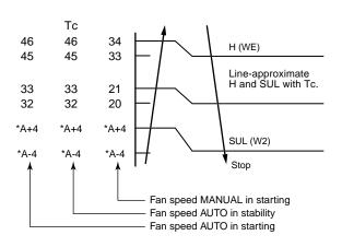
\* No limitation while fan speed MANUAL mode is in stability. \* A: When Tsc  $\geq$  24, A is 24, and when Tsc < 24, A is Tsc Tsc: Set value
