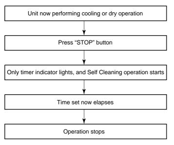
• During Self-Cleaning operations: The louver opens slightly. The indoor fan operates continuously at a speed of SL rpm.
