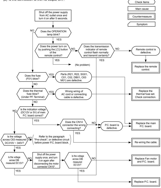
\* Be sure to disconnect the motor connector CN10 after shut off the power supply, or it will be a cause of damage of the motor.
